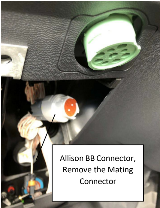
Figure 11 Allison BB Connector
