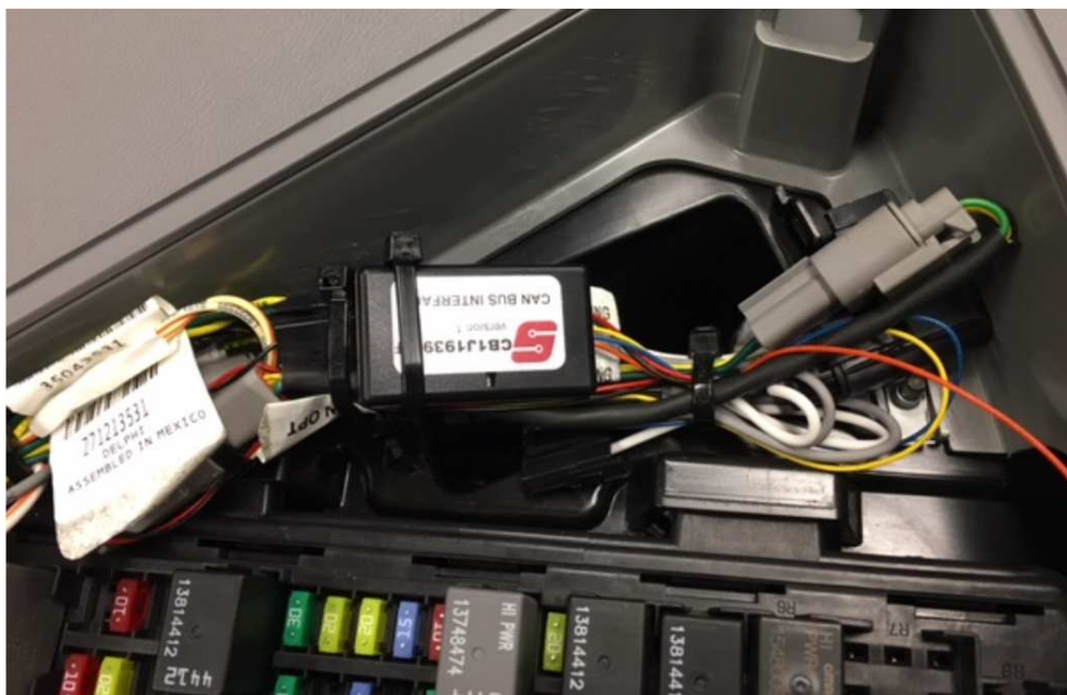
Fig. 45 CAN Bus reader installed
